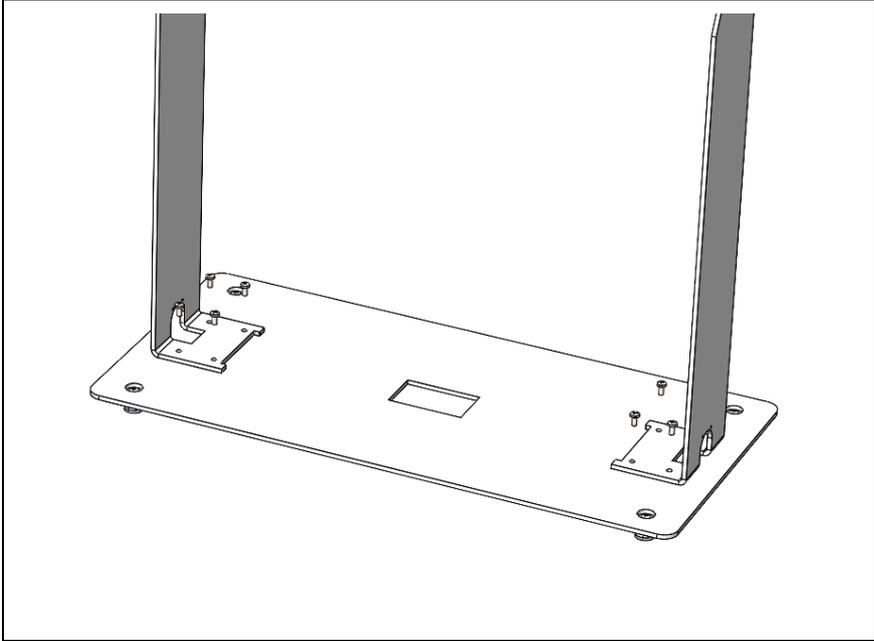
4. Connect the pillar to the bottom plate with 8 screws (**M6X12 MRT**)
