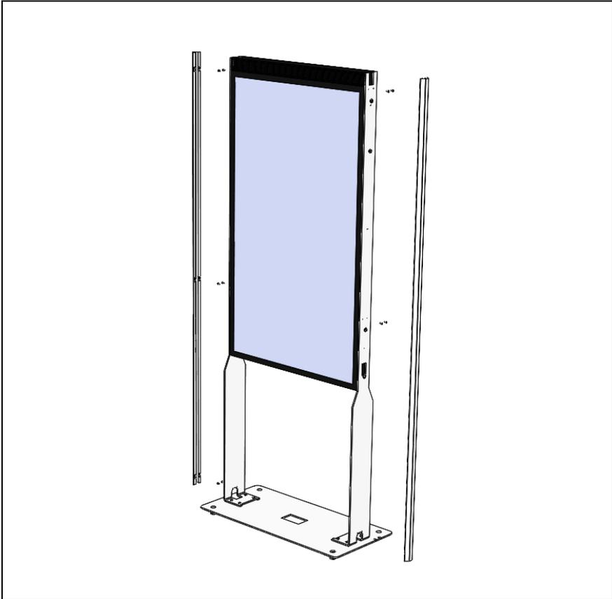
13. After connecting the cables the décor list can be mount on each side
