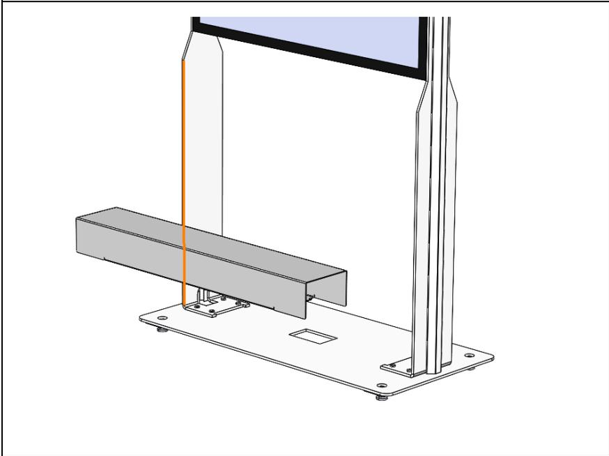
14. To hide all the cables and screws cover can be placed
