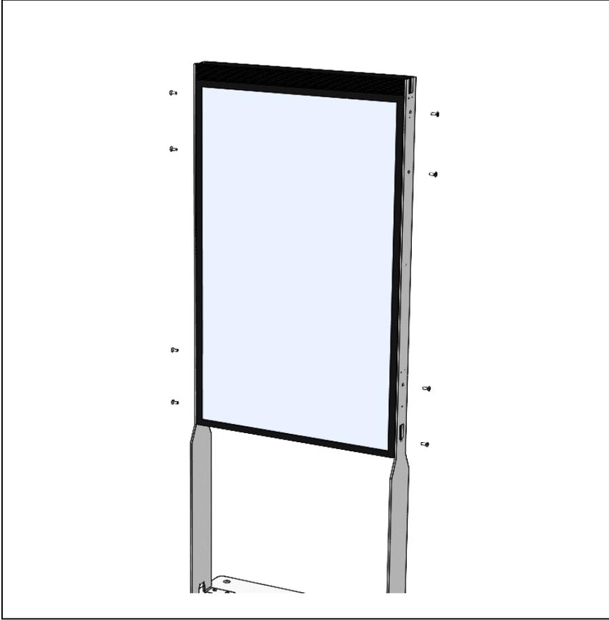
12. Screen can now be attached to the floor stand with 8 screws (**M8x20 MFX**)
